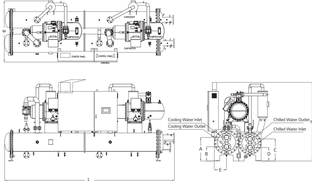
Tolerance : Chiller dimension ±50, Pipe Dimension ±30mm / Unit : mm
