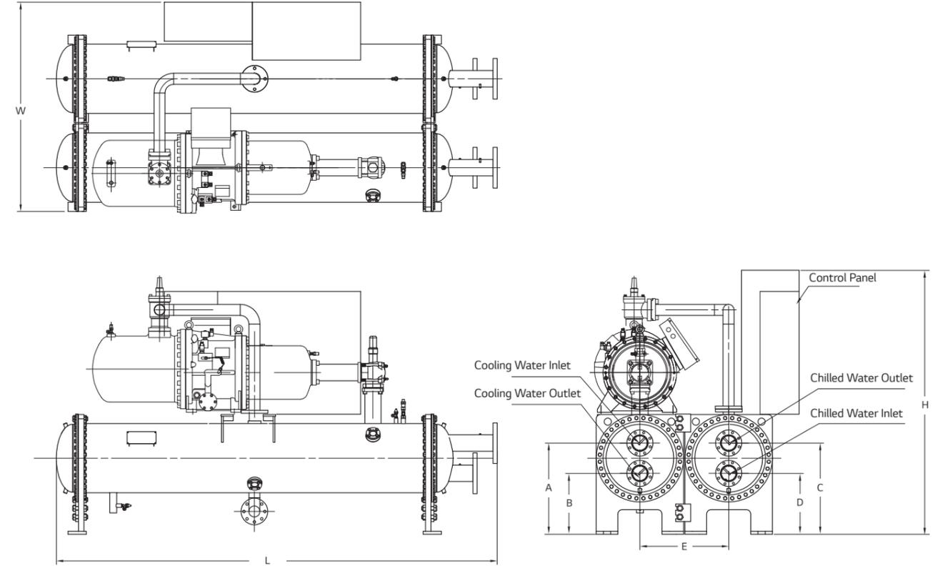
Tolerance : Chiller dimension ±50, Pipe Dimension ±30mm / Unit : mm
