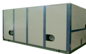
◆ Indoor Unit of an Evaporative Chiller Cooling Capacity Range: 433KW~2111KW Chilled water outlet temperature range: 5~20°C
